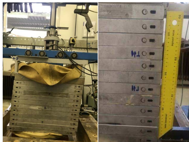
Figure 5. Deformed test specimen on the Large-Scale Triaxial test apparatus.
