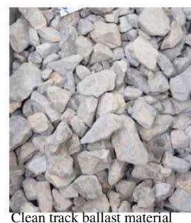
Clean track ballast material
