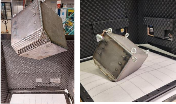
Figure 3. Impact test on non-woven on the smooth point (point s).
