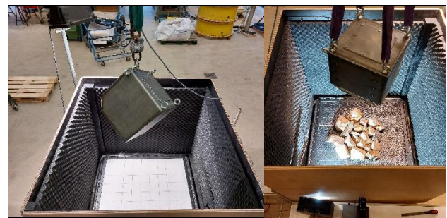
Figure 1. Setup examples with stone drops directly on a non-woven (left) and on a stone ballast layer (right). The stones were randomly placed.
