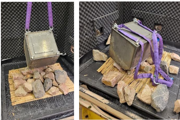
Figure 4. Impact test on ballast and reed. Block on rib.
