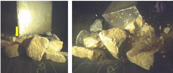
Figure 5. Test 136. Series 46 Flat side of block dropped on stones ballast layer and geotextile from 5 m. Start impact (left picture) and after impact (right). The arrow at the left picture indicates breakage of stones due to impact.
