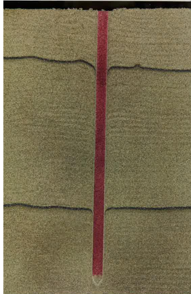
Figure 10. Cone penetration testing (after extraction of the penetrometer, the hole was filled with red sand).
