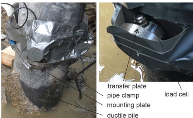
Figure 6. Measurement device mounted on Ductile Pile to investigate horizontal loads resulting from bracing effect.
