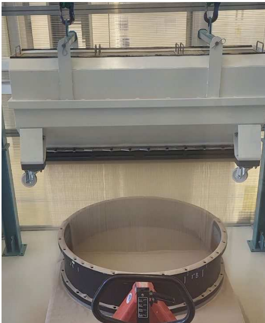
Figure 6. Sand-rainer; Sand-curtain; cylindrical test-box.
