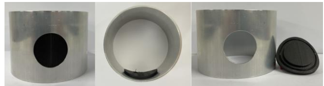
Figure 5: Trial of the lower part of the shaft showing the curved plug arrangement.
