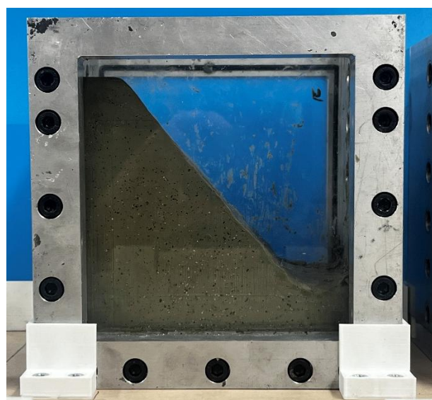
Figure 8. Example of completed soil model ready to test.
