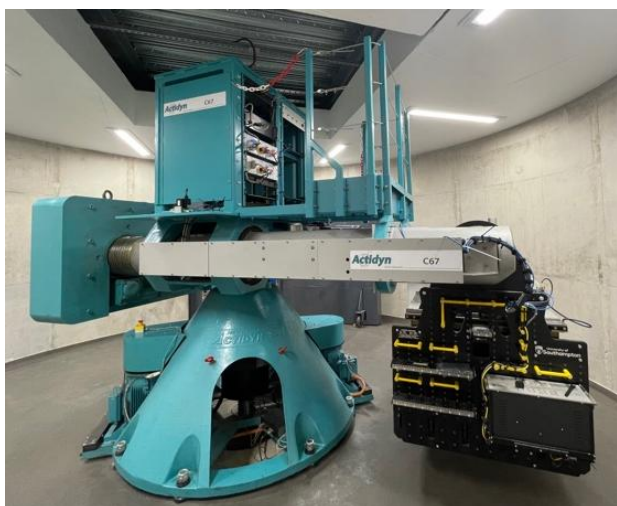
Figure 1. Actidyn C67 centrifuge at the National Infrastructure Laboratory, University of Southampton.
