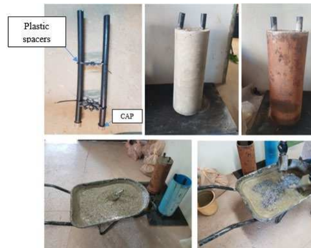
Figure 2. Piles constructed for physical model tests (concrete and steel pipe pile section), and concrete with and without steel fiber used as pile filled material.
