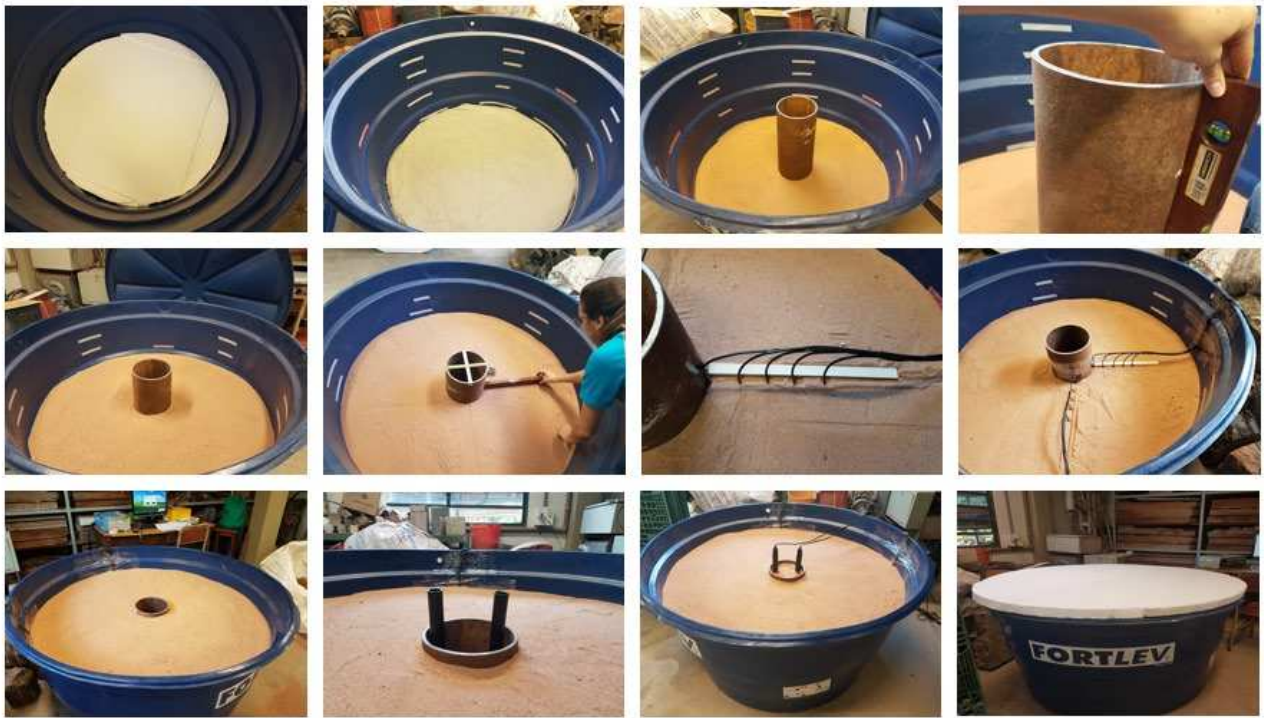
Figure 3. Test assembly steps for the tests in dry sand.
