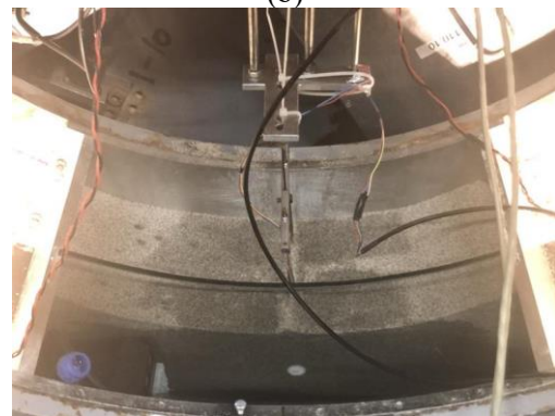
Figure 7. (a) The setup of the mini-drum interior (b) the schematic setup of the mini-drum interior (Wang et al., 2011), and (c) the setup of UHB model.
