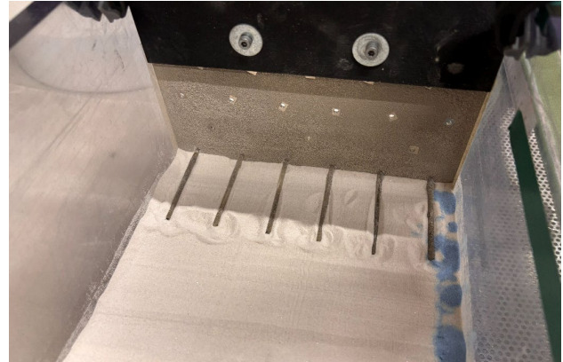
Figure 3: construction of the soil nail wall model using coated PMMA model nails
