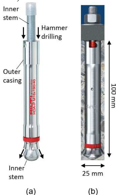
Figure 3 A Hilti HDA-P M10 anchor (a) before installation (b) after installation
