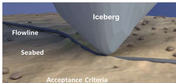
Figure 1. Expected flowline response on sand from impacts with free-floating icebergs
