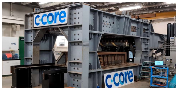
Figure 5. Completed RHITA Frame.
