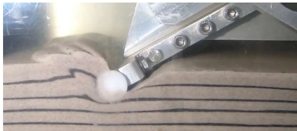
Figure 12. Post test of rapid inclined loading.
