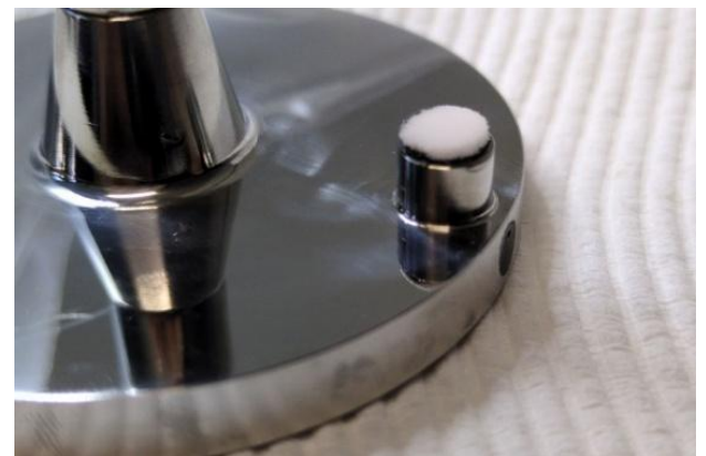
Figure 2. Close-up view of the top pore water pressure transducer located 5 mm above the top face of the anchor.
