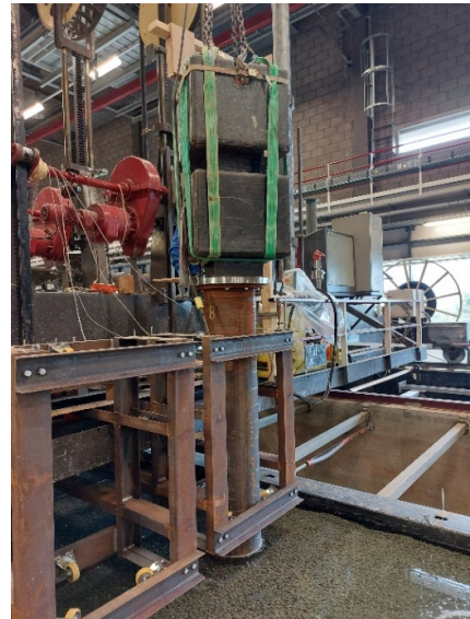
Figure 7. A photograph of the force-controlled pile penetration tests.
