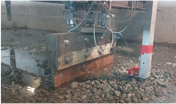
Figure 2. An exemplar image of the displacement-controlled plate penetration tests.
