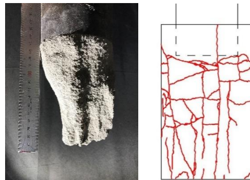
Figure 12. CASE 4 failure mode.
