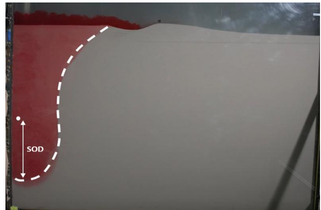
Figure 3-1. Picture of the jet pit in the tracer experiment, including jet position and schematics of stand-off-distance.
