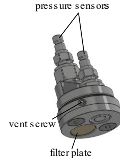
Figure 6. Pile tip with sensors and mounted filter plate
