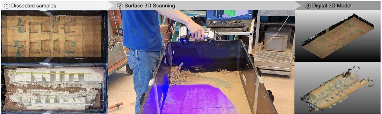
Figure 6. Measurement procedure after testing: dissecting soil samples, scanning soil surfaces, and analysis of 3D scan
