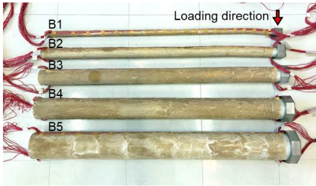
Figure 9. Pile model after loading.
