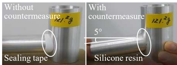
Figure 13. Connection between manhole and sewer pipe.
