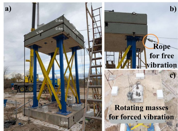
Figure 1. Overview of the EuroProteas experimental setup: (a) general view of the structure, (b) detail of the devices attached at the top of the structure for free vibration testing, and (c) rotating masses used to induce forced vibration.
