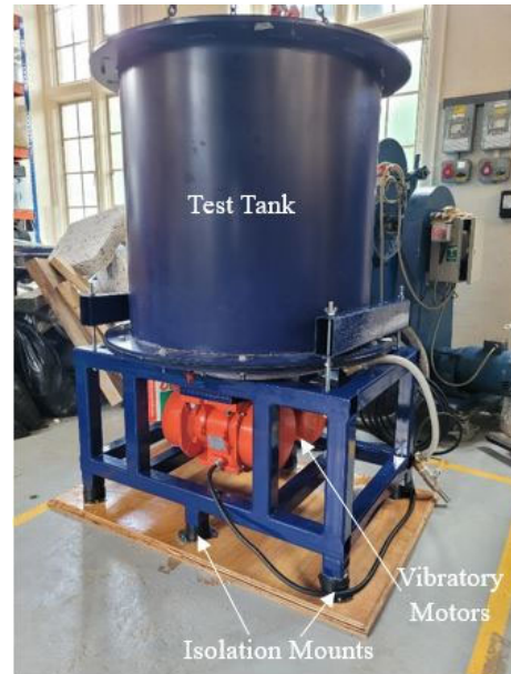
Figure 3. Sample preparation for saturated sand by means of reconstitution.
