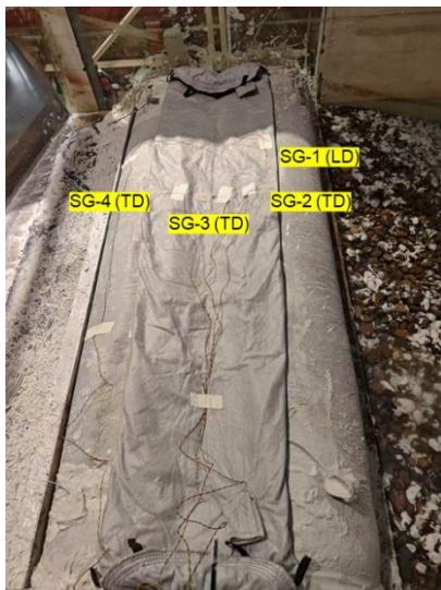
Figure 4. Strain gauge setup on the upper geotextile tube.
