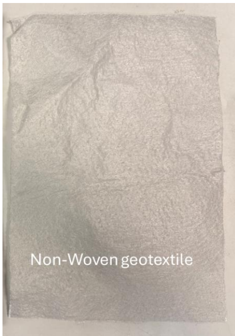
Figure 1. Non-woven geotextile used in the model tests.
