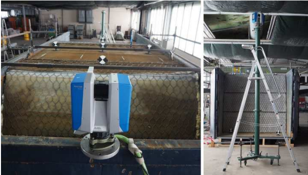
Figure 5. Zoller + Fröhlich Imager 5016 positioned on the upstream side (left) and on the downstream side (right).
