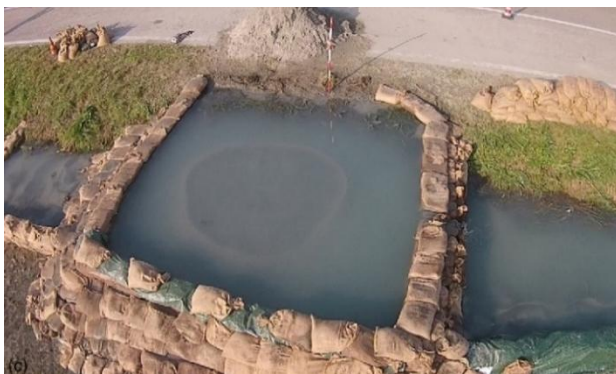
Figure 2. Sand boil along a stretch of the Po River (Italy) reactivated during the 2014 high-water event: the approximate diameter of the external sand volcano is 2.5 m (Marchi et al., 2021).
