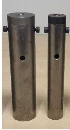
Figure 3. Model piles used in testing
