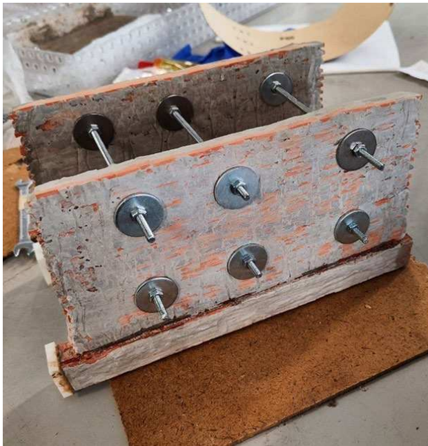
Figure 2 Side view of the GIANO-1 test structure before the installation in the centrifuge box.
