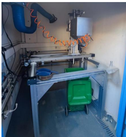
Figure 3. Automatic sand pourer at the University of Nottingham, University Park Campus, UK.
