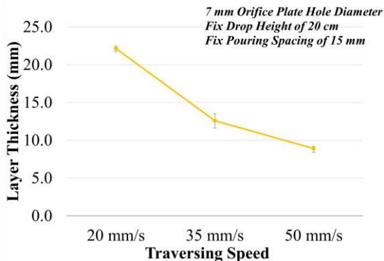
Figure 11. Change in the poured layer thickness for increasing traversing speeds.
