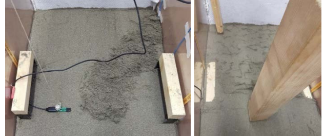
Figure 3. Exact placement of FDR probe with the aid of a plumb line and sand compaction with manual hammer. Wooden benches for the energy wall support are visible along the box sides.
