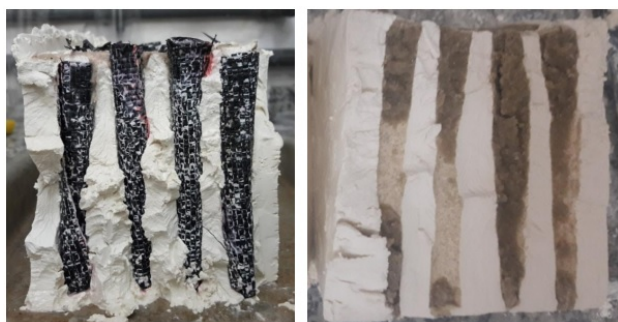
Figure 10 Exhumed soil container of: (a) Geotextile reinforced column pattern; (b) Conventional column pattern.
