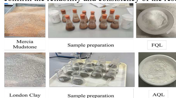
Figure 4. Sample preparation using quicklime for Mercia mudstone and London clay
