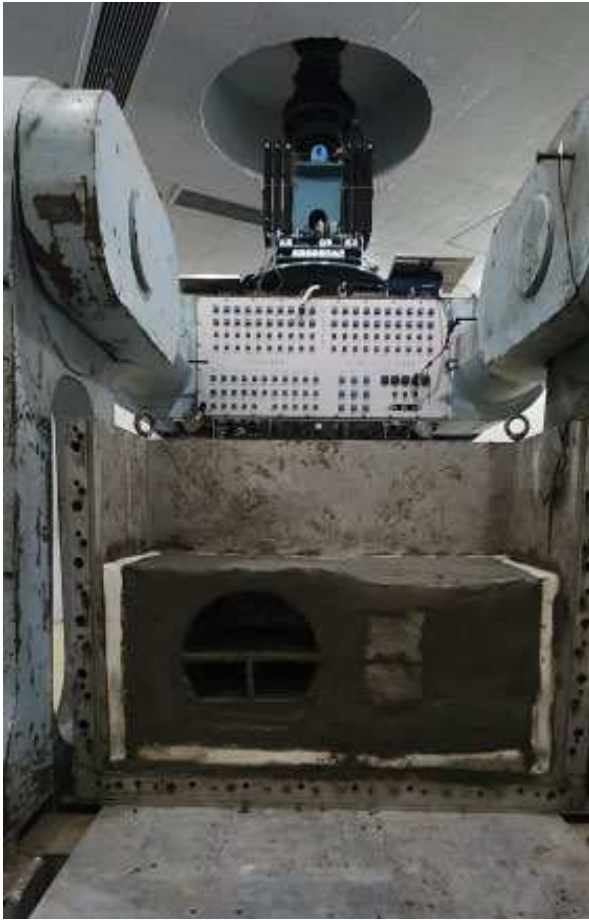
Figure 5. Vibration isolation wall arrangement.
