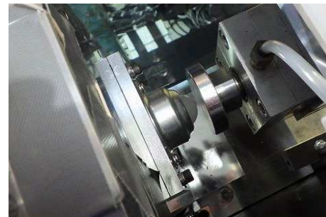
Figure 4. Inclined loading plate (left) and horizontal loading device (right).
