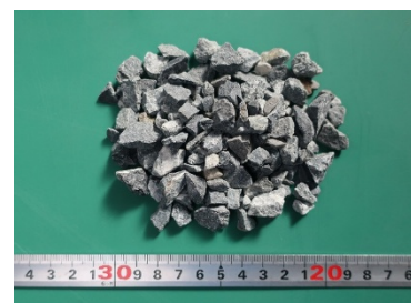
Figure 2. 10 mm crushed stones used for the reinforcing embankment.
