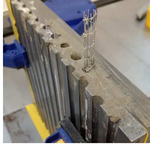
Figure 3. Mould adopted for the RC piles casting.
