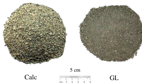
Figure 2. Photographs of the calcareous (left) and glauconitic (right) sands prior to testing.
