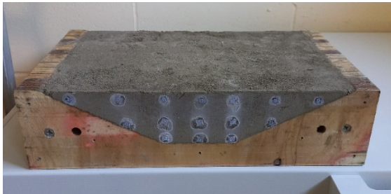
Figure 2. Model flood embankment prepared in the wooden mould
