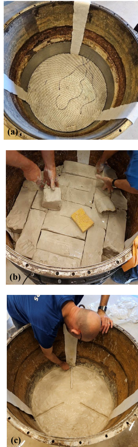
Figure 3. Preparation of the clay bed (each layer is inundated under water after installation of the horizontal sand seams). In (a) empty container with vertical drainage geotextiles; (b) blocks placed; (c) after tamping.
