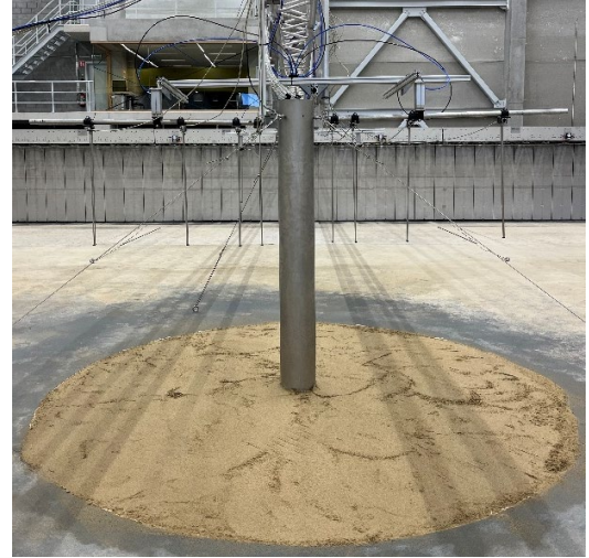
Figure 1. Overview of the experimental setup including the monopile, wave gauges, anchored ropes and filled central pit.
