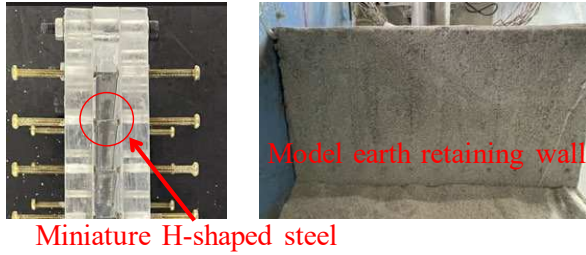
Figure 3. Model earth retaining wall.
