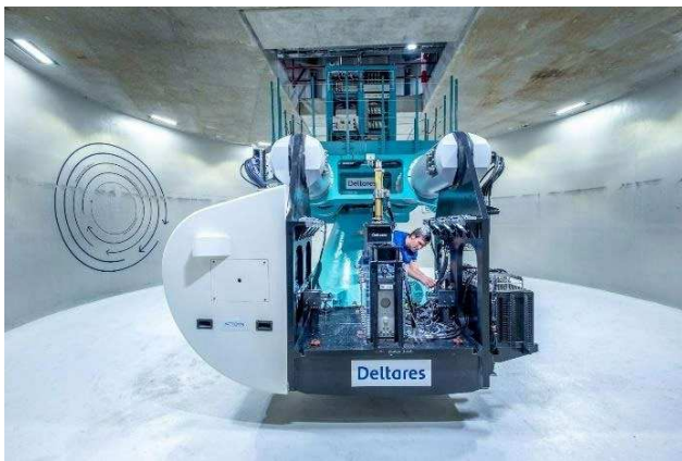
Figure 2. Side view of the beam GeoCentrifuge of Deltares.
