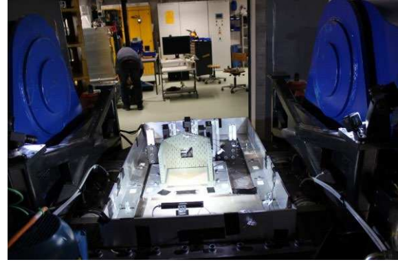
Figure 3. The ETH Zurich GCC beam centrifuge basket, showing the URM building specimen installed.
