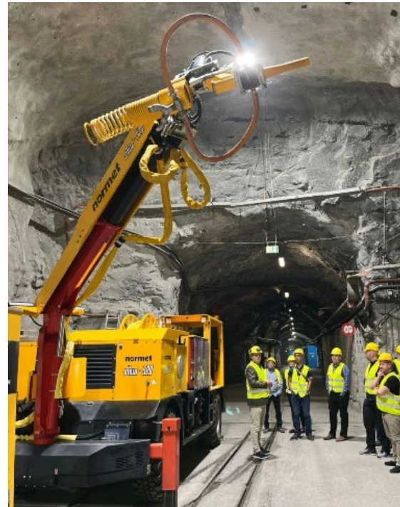
Figure 7. Example of a BEV for shotcrete application underground
