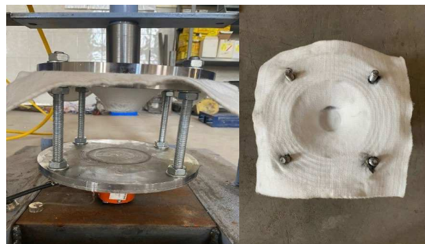
Figure 9. Tearing test apparatus.
