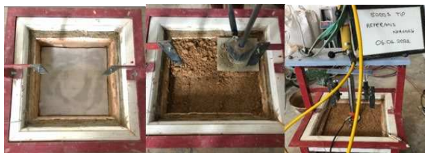
Figure 7. Experiment cell and instrumentations.
