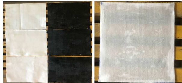
Figure 1. Geotextiles used in the study; reference, bitumen and resin impregnated ones, respectively.
