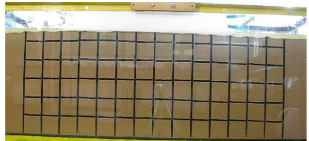
Figure 2. Experimental shaking table model before dynamic loading (View from camera No. 1)
