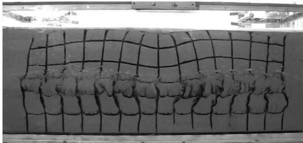
Figure 6. Qualitative displacements in the prepared sandy soil profile after application of base motion (test F4).
