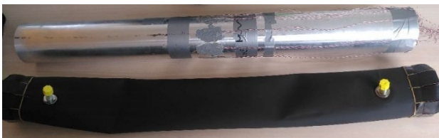
Figure 3: Photo of the aluminium pipe and internal pressurisation membrane
