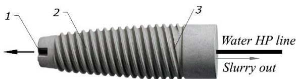
Figure 6. Ground implant with anti-plugging geometry, where: 1 – cross-slots; 2 – helical grooves; 3 – base.
