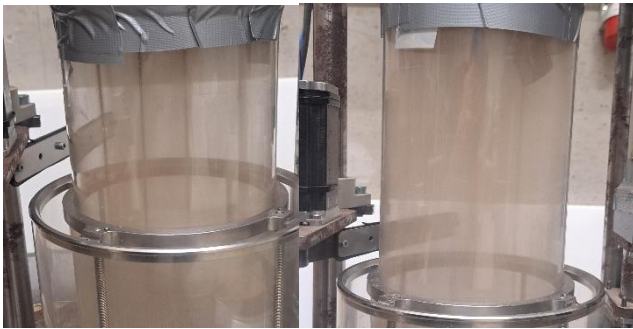
Figure 5. Examples of inhomogeneous flow (left) and homogeneous flow (right) after diffusor sieves.
