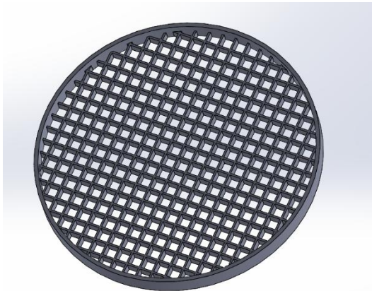
Figure 3. Model used for 3D-printing of diffusor sieves (7 mm mesh size).
