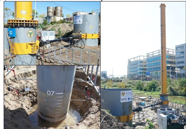
(c) Forced loading tests with superstructure
