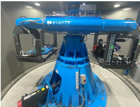
Figure 1. Mark III geotechnical centrifuge facility at TCU.
