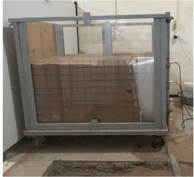
Figure 1. Glass box used for constructing the laboratory model.
